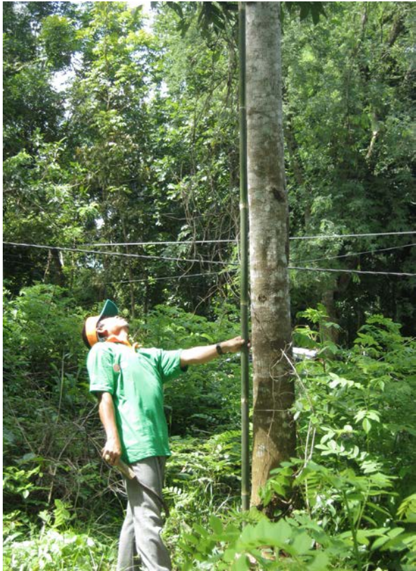
Picture 32. The practice of tree height measurements using simple tools (bamboo).
